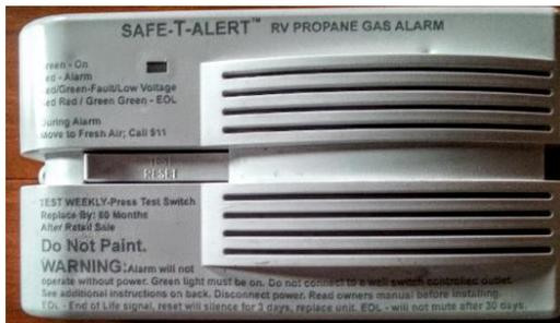
Each RV is equipped with a propane detector, which is always located near the floor. The alarm goes off whenever an increased propane emission (e.g. from the stove or oven) is detected. Please do not to place any objects near the propane detector to avoid false alarms.
