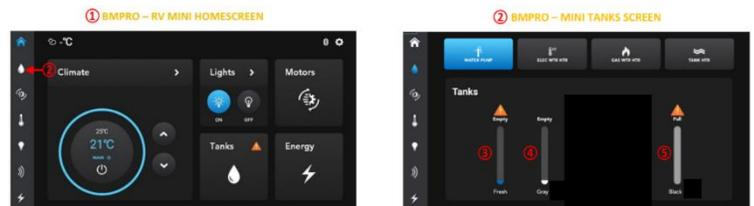
On the **BMP DISPLAY** touch the PAGE NAVIGATION button ① to get to the TANKS screen ①. Then you will find the levels of the FRESH ②, GREY ③ and BLACK ④ tanks.
