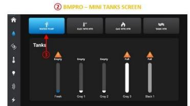
On the **BMP DISPLAY** just touch the WP button **d** to turn on or off the water pump.
