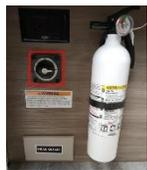
The main switch for turning the coach battery on and off is located directly next to the side entrance door at floor level. This switch allows you to turn the 12V battery, providing power to the motorhome's living area, on and off. If none of the 12V appliances in the motorhome is receiving power, it is possible that this switch was accidentally turned off. Please check if this is the case and turn it back on if required (ON position).
