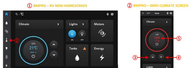
On the **BMP DISPLAY** touch the MAIN A/C button **a** to get to the AC screen **1**. ROOM **2** shows the current room temperature. The desired temperature SET **3** is set using the UP **6** and DOWN **7** buttons. These buttons are also used to select the MODE **4** and speed of the AC-FAN **5**.
