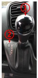
For driving in mountainous terrain and on routes with a lot of speed changes we recommend using the TOW/HAUL function. It prevents the transmission from shifting to the highest gear, gives the vehicle some extra power when going uphill and increases the brake force when going downhill to reduce the risk of overheating brakes. Select the function by pressing the TOW/HAUL ② button.
